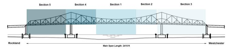
Tappan Zee Constructors (TZC) began dismantling and removing the Tappan Zee Bridge's main span in 2018 by dividing the steel into five discrete sections. The public can observe the operations with the project's <u>tower webcam</u>.
