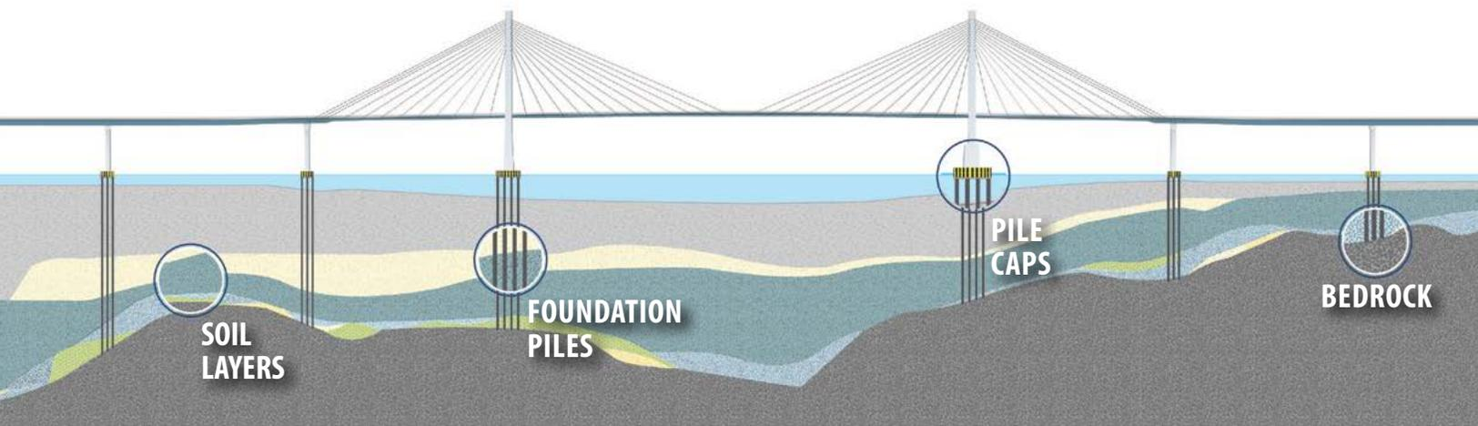
⤵ The placement and length of each pile is carefully calculated based on the project team's pile load tests and geotechnical investigations, which detailed characteristics of the layers of sediment and bedrock.
