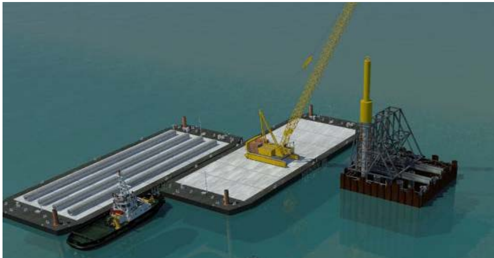
B. Install Pile template on sheet piles and drive piles
