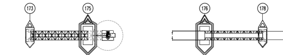
DISMANTLING CANTILEVER SPAN 4600 RINGER ON BARGE 65T HYDRO (2X) DEBRIS BARGES
