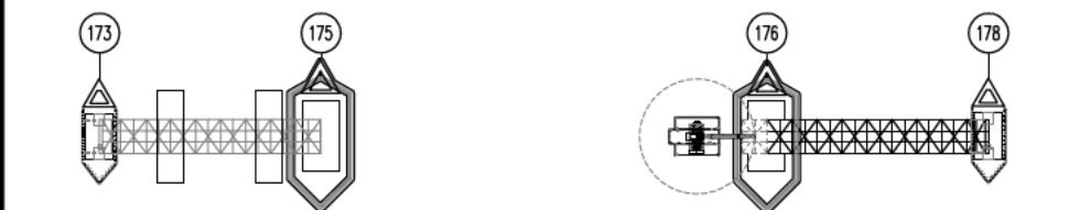
LOWERING ANCHOR SPAN 65T HYDRO 300T LR1300 (2X) DEBRIS BARGES
