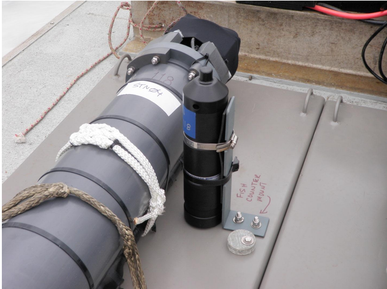
Figure 16. Acoustic recorder (gray) and VR2W 69 kHz Acoustic Monitoring Receiver (black) at Station 4 before deployment.
