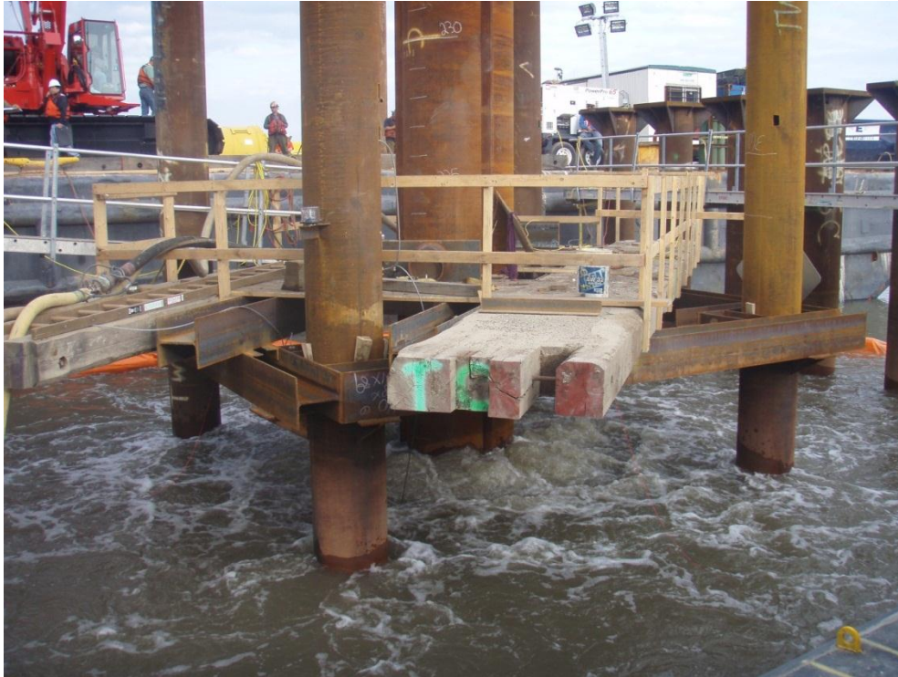
Figure 4. Base of Test Pile 1A showing air bubbles from the Unconfined Single-Tier Air Bubble Curtain, 5 May 2012.
