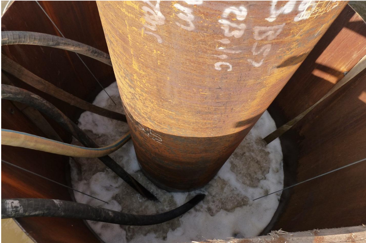
Figure 6. Photo inside the isolation casing at Test Pile 2B showing the air bubbles from the Isolation Casing and Bubble System, 16 May 2012.
