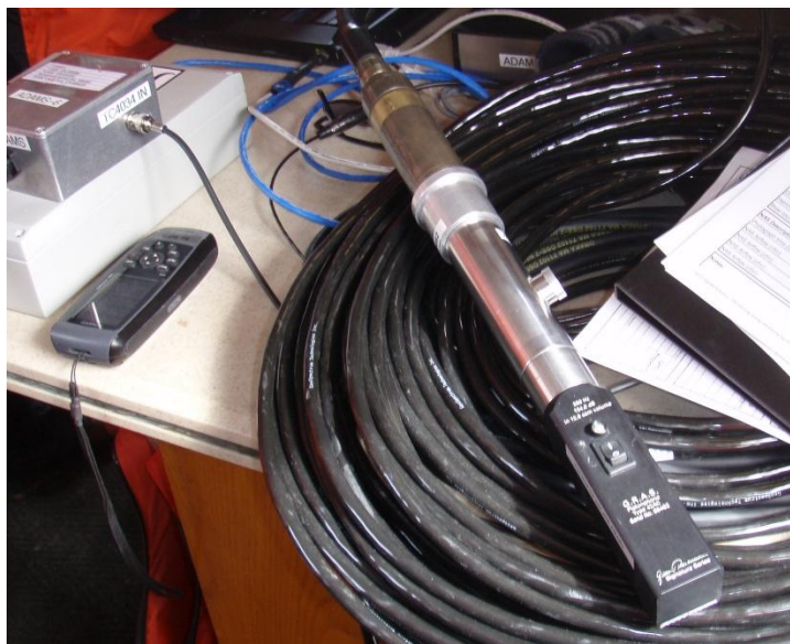
Figure 14. Example of a GRAS pistonphone calibrator on a RESON TC4032 hydrophone. The RESON hydrophones—TC4032 and TC4034—used for short-range monitoring, and the M8E and M8K hydrophones, used for long-range monitoring, require different adaptors (not shown).
