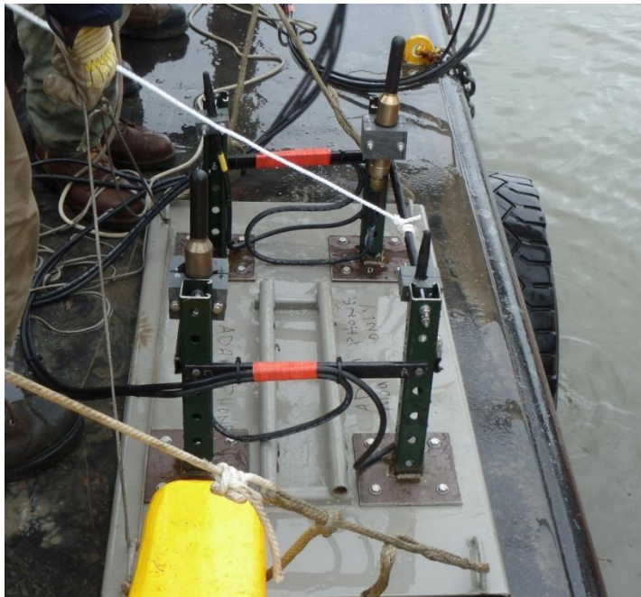
Figure 11. The hydrophone mounting plate prepared for deployment for short-range hydroacoustic monitoring. The smaller RESON TC4034 low-sensitivity hydrophones are top left and bottom right; the larger RESON TC4032 high-sensitivity hydrophones are bottom left and top right. Each pair of hydrophones is connected to a JASCO ADAMS for monitoring in real time and recording.
