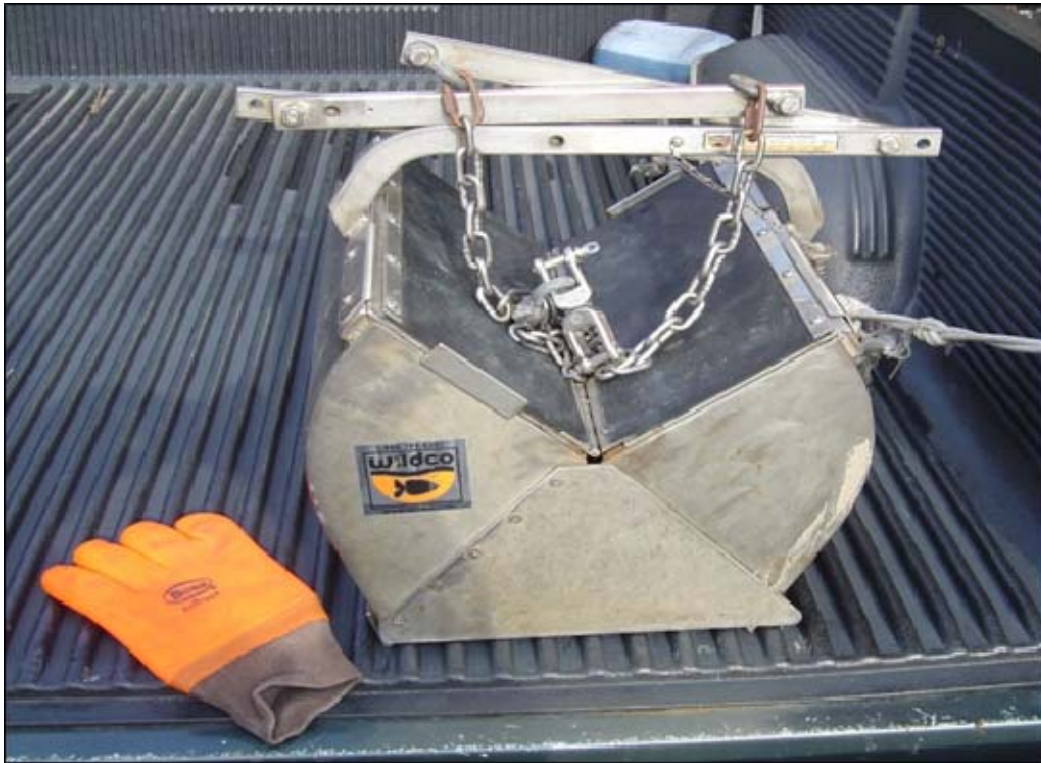
Photo F-1-7 A Van Veen Grab Used for Benthic Sampling. Note glove for scale.
