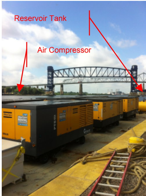
Figure 1. Air Compressors and Reservoir Tanks on the Air Compressor Barge
