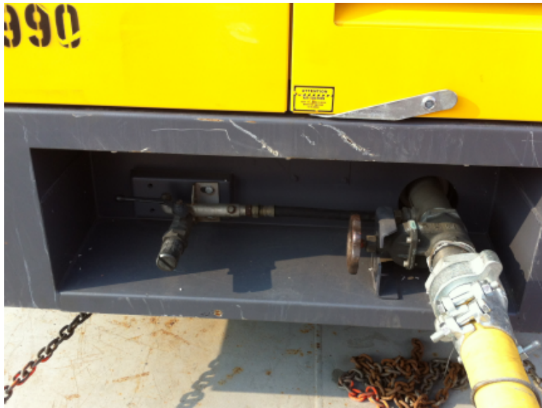
Figure 7. Valve at the Air Compressor Outlet to the Reservoir Tank
