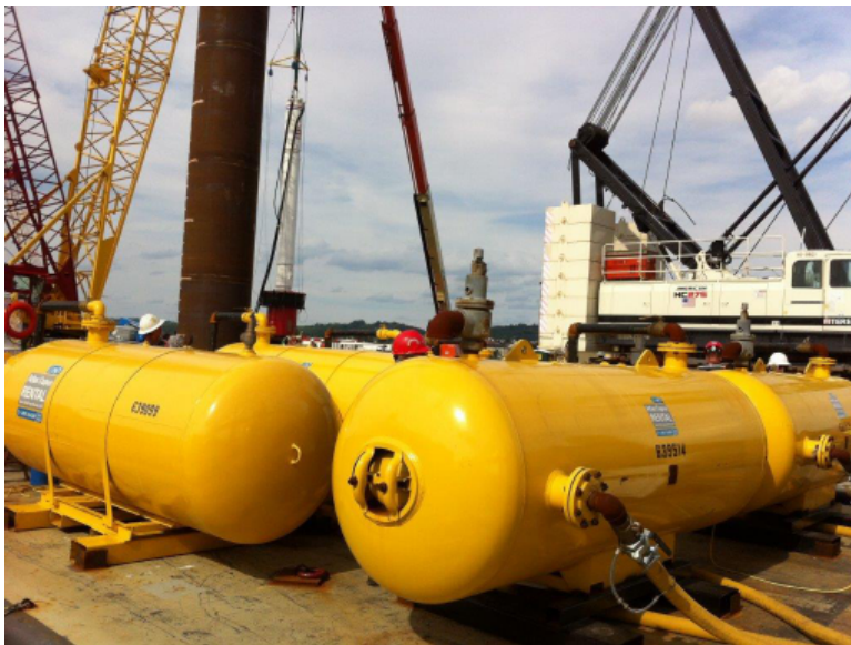
Figure 2. Reservoir Tanks on the Air Compressor Barge
