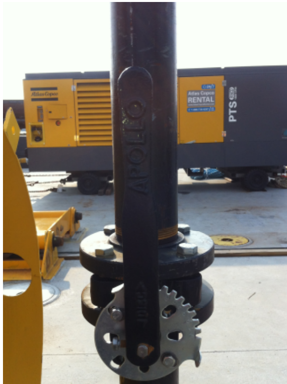
Figure 9. Valve at the Outlet from the Reservoir Tank to the Bubble Curtain
