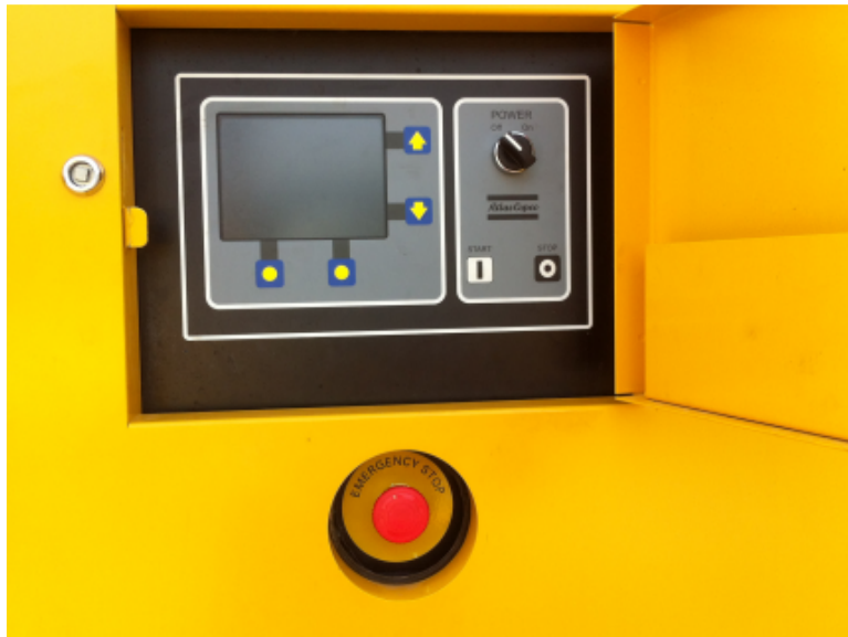
Figure 10. Air Compressor Controls
