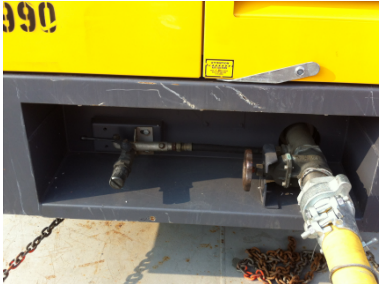
Figure 6. Valve at the Air Compressor Outlet to the Reservoir Tank
