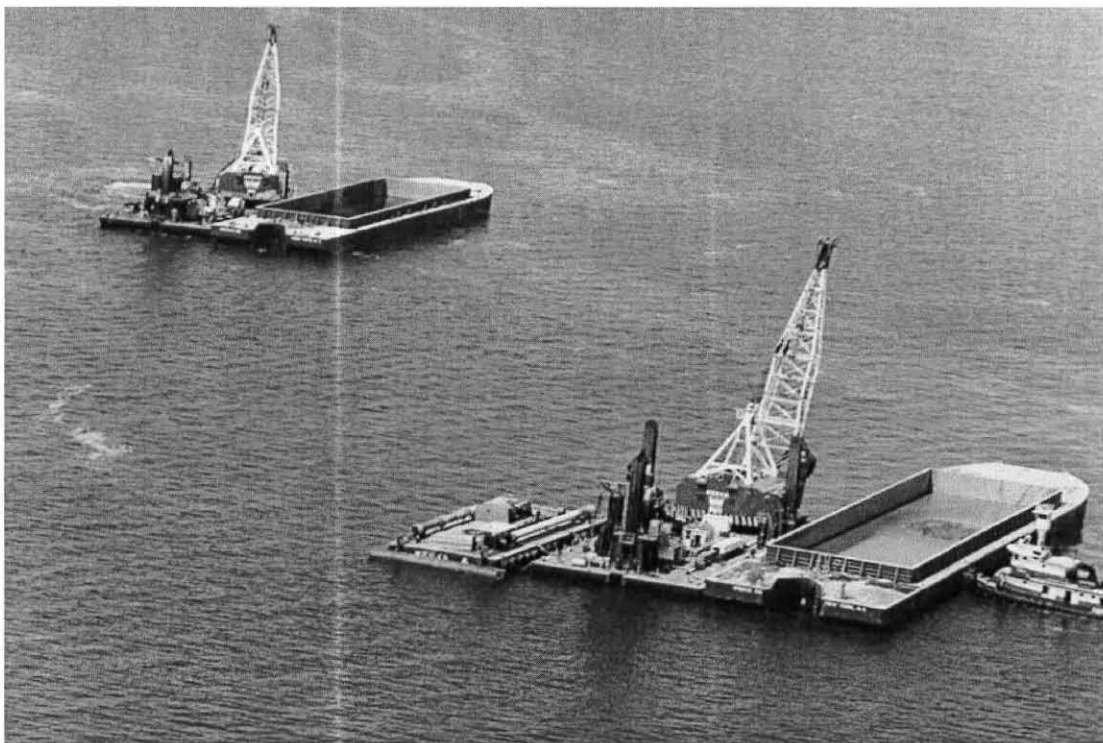
DREDGE 551: 25 CY BUCKET. 1,742 INSTALLED HP.
