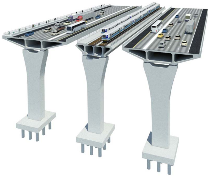
Option 1 – Single Level CRT Center Three Structures Two highway/BRT (HOV/HOT or Busway) structures with a central CRT structure
