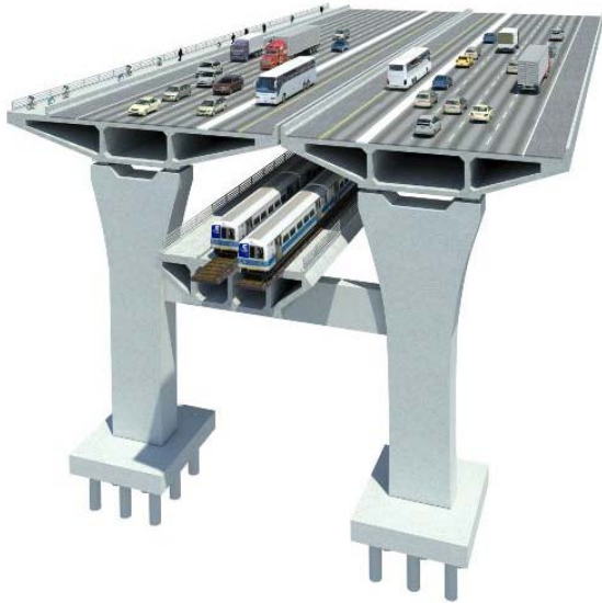
Option 4 – Dual-Level CRT Center Stacked Option One Structure Two highway/BRT (HOV/HOT or Busway) decks above a central CRT deck on a composite single structure
