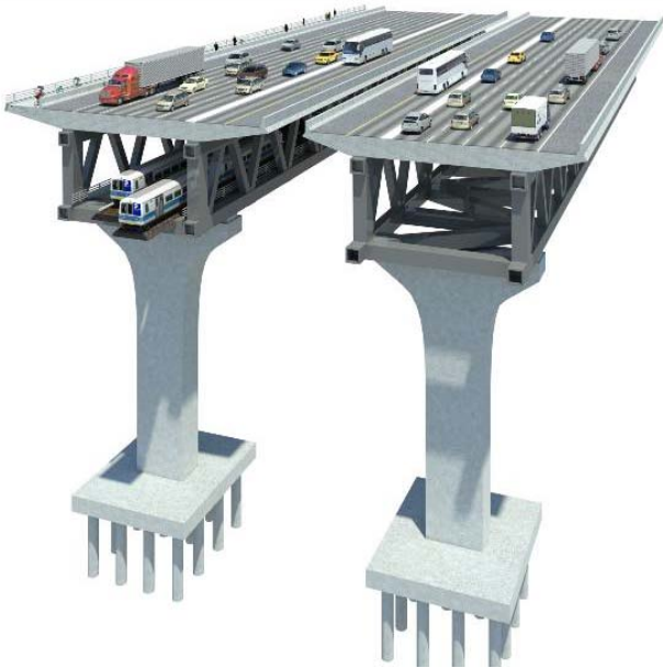
Option 5 – Dual- Level CRT North Two Structures Two Dual-level structures with highway/BRT (HOV/HOT or Busway) decks above an CRT below on the North
