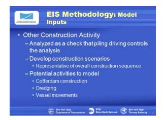
Slide 37. In addition to estimating sound levels from pile driving, we also will predict levels generated by other construction activities such as vessel movements and cofferdam construction.
