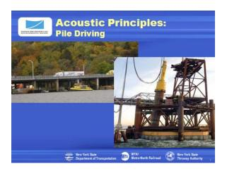
Slide 23. In the vicinity of the existing TZB, there are many existing sources of noise including ship traffic and vehicle traffic. Noise from the bridge itself is transmitted as vibration through the bridge supports and into the water column, where it becomes underwater noise. Construction-related noise would be in addition to this existing noise.
