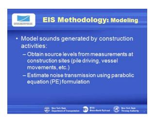
Slide 35. The expected modeling process was described. The first step in the process of estimating the project's acoustic footprint is to obtain data from actual pile-driving sites. That data will enable us to estimate the source strength of the pile driving. The next step is to estimate the transmission of sound though the Hudson River using highly sophisticated mathematical modeling techniques.
