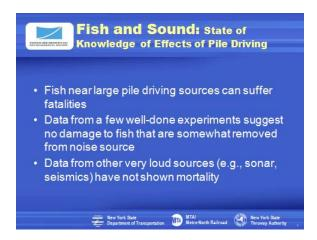
Slide 30. Experience in other projects has shown that fish in close proximity to certain pile-driving operations can suffer fatalities as a result of underwater noise. Experiments suggest that fish need to be very close to the source. Obtaining this distance through experimentation using actual pile-driving has been problematic so there is little actual data. Data from experiments using other very loud sources (such as sonar) that can be deployed in a lab setting have not shown mortality.
