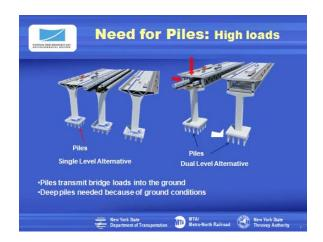
Slide 8. Two of the six options were shown to explain the primary components of the replacement structure, which include decks, piers, and foundations (pilecaps and piles).
