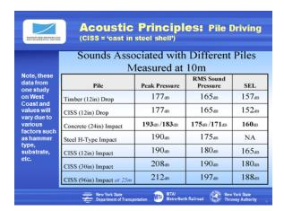
Slide 25. The noise generated by a pile as it is driven will vary based on the type of pile, how it is driven, the depth of water, the energy of the pile driver, the type of river bottom, and several other factors. In short, there is no single noise level that will predictably occur. However, CALTRANS has carried out extensive monitoring programs in an attempt to develop some typical ranges, and they have found that SELs from pile driving might vary from 152 dB to 188 dB.
