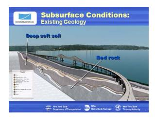
Slide 9. Various substrate components are found beneath the Hudson River bed, with rock at depths ranging from 200 to 700 feet below the mudline. As the substrate is generally soft and rock is deep, extensive piling would be required to support the replacement Tappan Zee Bridge (TZB).
