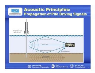
Slide 24. Noise travels from a source to a receiver over several paths. There is the direct path that sound takes between the two points. Sound can also bounce off the water surface and the river bottom, just like sound echoes off walls in a room. There is another way sound can travel: vibrations can travel through the ground, and then be radiated from the river bottom, much like the loud bass sounds you might hear from a neighbor's stereo.
