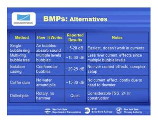
Slide 44. This slide illustrates the noise reduction benefits that can be expected from various BMPs based on data obtained from other bridge construction sites.
