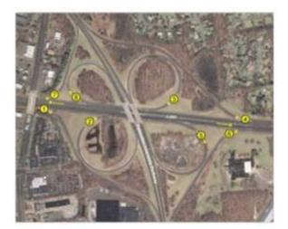
Auxiliary lanes separate the weave/merge operations in a separate roadway parallel to the highway. Traffic analyses show their effectiveness:
