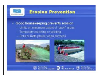
Means of preventing erosion include limiting the size of active work areas, stabilizing exposed areas using temporary mulching or seeding, or use of methods such as rolls or mats to cover disturbed areas. The photo on the left shows the application of temporary seeding using the hydroseeding technique. The photo on the right shows a typical installation of an erosion control mat .
