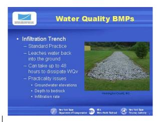
Infiltration trenches are another standard practice. They are essentially "containers" in the ground that collect stormwater and dissipate it into the surrounding soil. The areas in which infiltration trenches are applicable are not as wide-ranging as those for stormwater ponds and wetlands because there are often issues that prevent sufficient flow of water into the soil, such as the presence of groundwater, rock, or relatively impermeable soils (such as clay).
