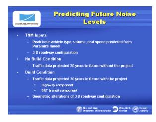
Traffic noise model inputs to be considered under the future no build and build conditions.
