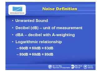
This slide defines noise, presents units of measurement, frequency weighting (A-weight) that best fits human perception of noise, and mathematical relationship applicable to adding and subtracting noise from different sources.
