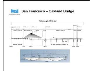
This slide shows both a side view and a cross section of the east spans of the SFOBB.
