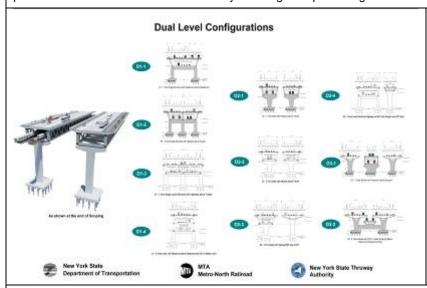
This graphic was used as a basis to discuss possible bridge configurations possible for a dual level bridge.
