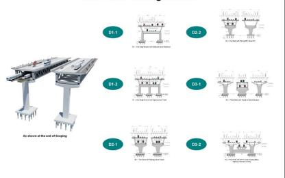
This graphic was used as a basis to discuss possible bridge configurations possible for a dual level bridge. The graphic shows seven possible configurations. A number of additional configurations were developed during discussions which will be added to the graphic for the next meeting.
