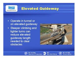
Because the LRT vehicles can climb grades up to about 6% and make tighter turns than RRT or CRT vehicles, when they must go over an obstacle they can do so in less distance, reducing the amount of elevated guideway and saving money.
