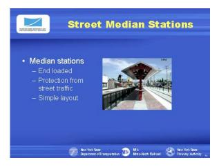
As mentioned earlier, street median stations are usually end loaded. This one features a railing so riders cannot step into a moving traffic lane on the back side of the platform.
