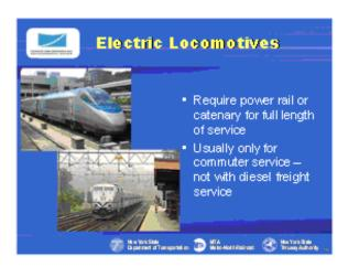
Slide 14: Where freight trains are not an issue, an all electric option is the electric locomotive. The top picture is the Amtrak Acela high speed locomotive.
