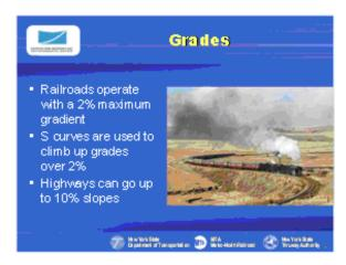
Slide 7: In addition, rail systems cannot climb the sort of steep grades cars and buses can, so they have to resort to several strategies when a steeper slope is involved. First, the tracks can be placed in an "S" curve to increase the distance, but this takes lots of space.
