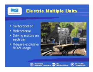
Slide 15: Then, there are "self propelled" commuter rail cars, called EMU's for electric multiple units. The picture shows a Metro North train at a station platform and you can see the third rail which provides power to these trains.
