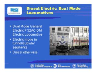
Slide 12: As far as locomotives go, they come in a number of choices including diesel/electric dual mode that can operate on third rail power in tunnels and terminals and diesel elsewhere. This saves the cost of electrifying miles of track where diesel operations are feasible.
