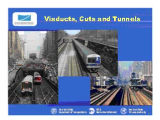
Slide 8: Or they can be put on elevated structures, or in open trenches or even tunnels to keep the tracks maximum grade under 2%. That is why some rail lines have so many more tunnels, open cuts and bridges than roadways in the same corridor.
