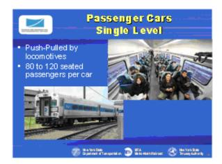
Slide 16: The next piece of equipment is the passenger car. This is a typical single level passenger car. These cars are designed to give everyone a seat, and can handle between 80 and 120 passengers depending on their interior layout.
