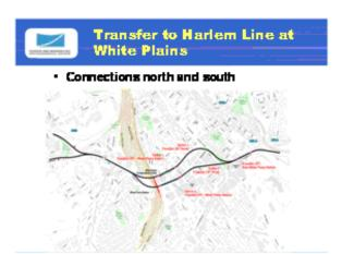
Slide 33: The Harlem Line could not be directly accessed because of the relative elevations of the Tappan Zee and Hudson Lines (the Hudson Line is elevated and the Tappan Zee CRT alternative would be in tunnel) and the presence of environmentally sensitive uses.
