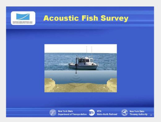
The slide shows a typical vessel used to conduct a bathymetric survey. Bathymetric surveys measure the depths of a body of water.
