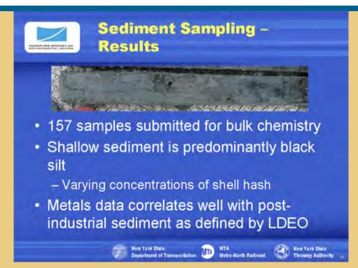
A typical sediment sample retrieved by vibra-coring methods. 157 one-foot-long sediment samples were generated from the 38 cores collected near the Tappan Zee Bridge. These samples were sent for laboratory analysis.
