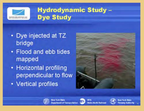
The objective of the dye study whose was to provide further data for calibration of the multi-dimensional hydrodynamic mathematical model. Dye was injected into the river during both flood and ebb tidal conditions. Dye concentrations were then monitored over a period of hours to obtain an understanding of the dispersiveness of the Hudson River at the Tappan Zee Bridge.
