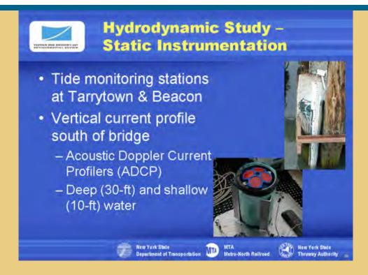
This hydrodynamic survey program relied heavily on the use of acoustic Doppler Current Profilers (ADCP) for data acquisition. The ADCP is a sophisticated and expensive instrument that measures water velocities across a column of moving water.
