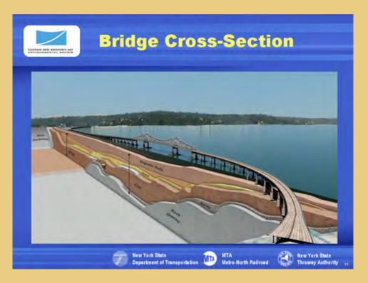
This cross section of the river illustrates geological conditions at the site of the Tappan Zee Bridge. The upper layer of material consists of organic soils, which are of principal interest from the perspective of assessing environmental impacts.
