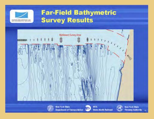
This typical far field, single beam bathymetric map is clearly less detailed than maps generated from the multi-beam survey system.
