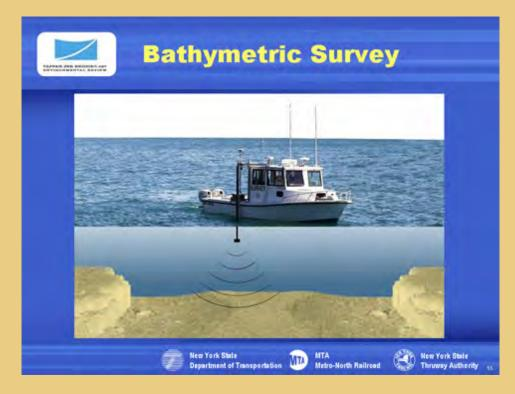
A typical survey vessel has antennae that receive GPS signals from satellites and shore-based stations. An acoustic sounder is mounted off the side of the survey vessel.
