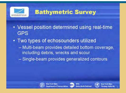
Two types of acoustic systems were used to generate bathymetric maps for the Hudson River program: a multi-beam survey, which was used to generate very detailed maps in the immediate bridge vicinity, and a single beam survey system, which generated maps in the far field.
