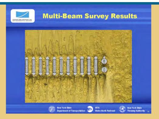
Scour maps due to river flows are clearly visible on this map, which illustrates typical results of the highly detailed multi-beam survey conducted in the immediate bridge vicinity.
