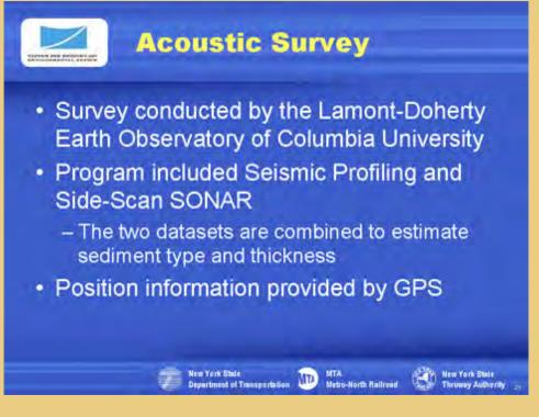
The acoustic profiling surveys were conducted by Lamont Doherty Earth Observatory to obtain an understanding of sediment depositional history in the vicinity of the Tappan Zee Bridge.
