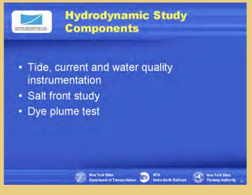
The hydrodynamic studies included tide-current-water quality measurements, a salt front study, and a dye plume test. The purpose of the program was to obtain data for calibration of a multi-dimensional hydrodynamic model that will be used to assess the impacts of bridge construction.
