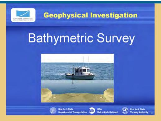
A typical vessel used to conduct a bathymetric survey. Bathymetric surveys measure the depths of a body of water.
