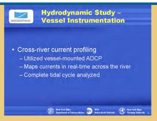
A vessel-mounted ADCP also was employed and mapped currents in real time across the river during a complete tidal cycle.
