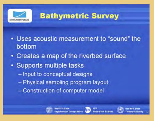
To measure the depth of the river, we used an acoustic system that "sounded" the river bottom. The result is a map of the river bottom. The bathymetric data will serve as input to bridge conceptual designs, assist with the layout of ecological and geophysical sampling programs, and will also provide input to a mathematical model being developed for the study.
