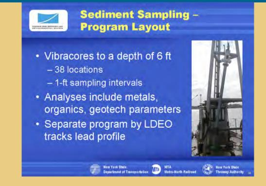
Sediment samples were obtained at 38 locations along the alignment of the existing bridge and along the potential alignment of a new bridge (samples obtained near the existing bridge are sufficient for the evaluation of the rehabilitation alternative). The chemical analyses were for metals, organics and geotechnical parameters.
