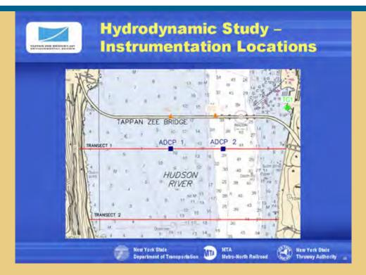
This slide shows where the fixed station ADCPs were located and the location of the transects followed by the vessel-mounted ADCP.
