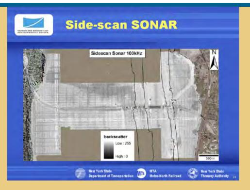
This side scan SONAR map of the vicinity of the Tappan Zee Bridge shows areas of high reflectivity (areas where surficial sediments are relatively coarse) and areas of low reflectivity (fine grained sediments).
