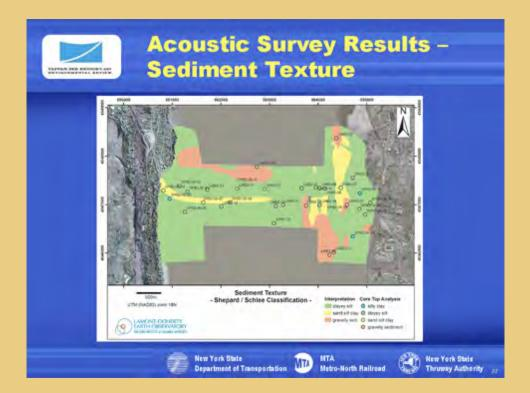
Illustrated here are surficial sediment texture classes, in the Bridge vicinity, as determined by the LDEO side scan SONAR survey and verified by a series of sediment samples taken by LDEO.
