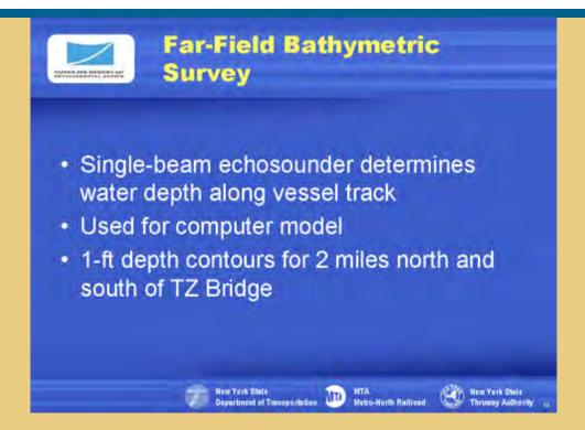
Far-field bathymetric surveys mapped the depths of the Hudson River from two miles above to two miles below the Tappan Zee Bridge.
