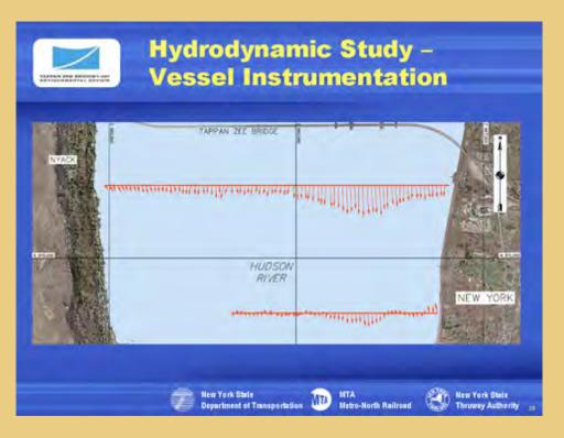
This typical image generated by the vessel-mounted ADCP shows that currents are strongest in the center channel and weakest near the river shorelines as would be expected.
