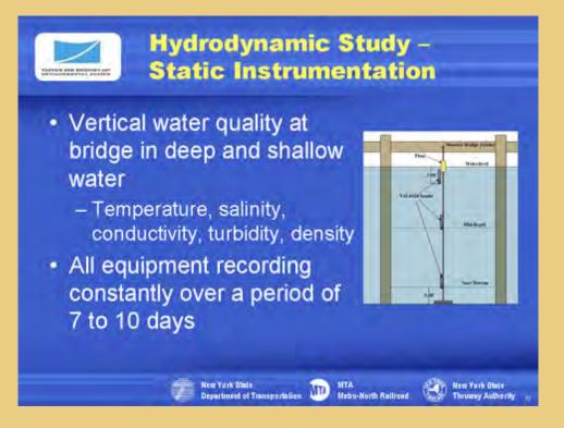
Fixed water quality sensors also were place in the river in deep and shallow water. The parameters measured included temperature, salinity, conductivity, turbidity, and density. All fixed station equipment recorded continuously for 7 to 10 days.
