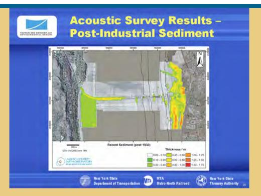
The estimated depth of recent sediment deposits in the Tappan Zee Bridge vicinity shows relatively thin (less than one foot thickness) deposits along the west shoreline area. Recent sediment deposits along the existing bridge alignment also are thin. Thicker, industrial era deposits occur on the east side of the river near Tarrytown. These deposits can be accounted for by streams discharging into the Hudson and also as a result of dredging activity.
