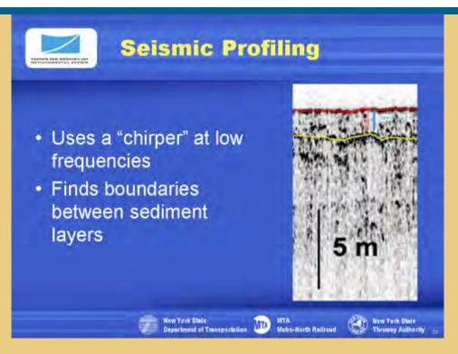
This illustration of the output of a typical sub-bottom profiling scan, and highlights the estimated boundary between recent and historic sediment deposits.
