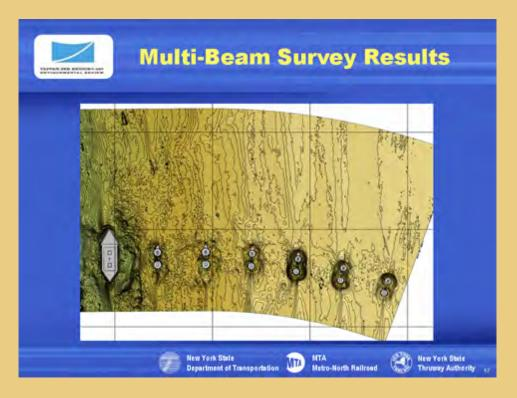
Scour marks are less pronounced in this map, which also illustrates results of a multi-beam acoustic survey.
