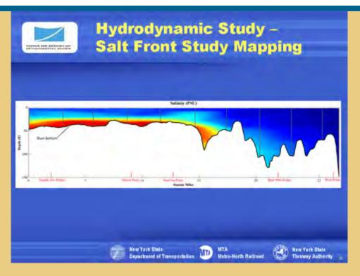
The position of the salt front, as measured during the salt front survey, shows that the salt front did not penetrate up-river beyond approximately mile point 43. The stratification between dense salt water and freshwater was highly discernible in the survey results.
